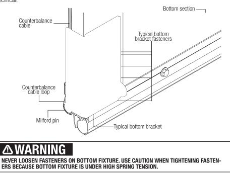
Inspect the cables. The cables should be tight and secured to the bottom fixtures. The cables should not rub against the door, track or any other objects. Cables with frayed or broken strands should be replaced by a trained door system technician.
